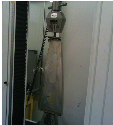
Fig. 5: Specimen under tensile test
